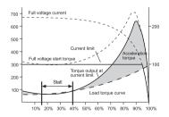
Start current can be estimated based on previous experience, or the motor and load speed/torque curves can be analysed for a precise calculation.
